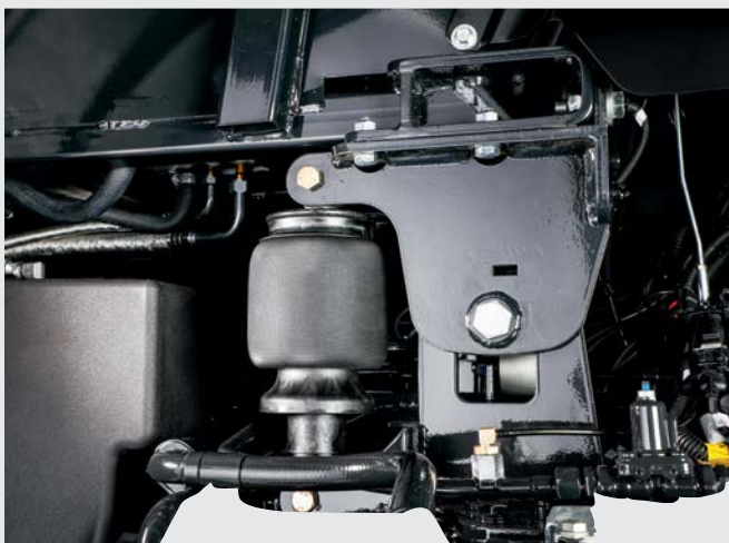
↑ Pneumatic cab suspension for a smoothest ride.
