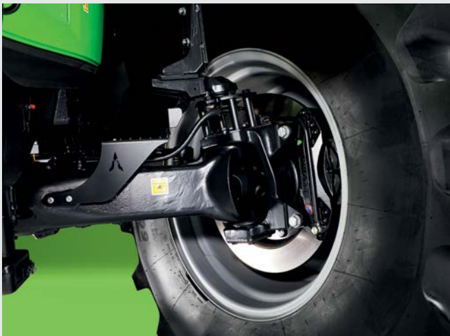
↑ Dry disc brakes for maximum brake performance.
