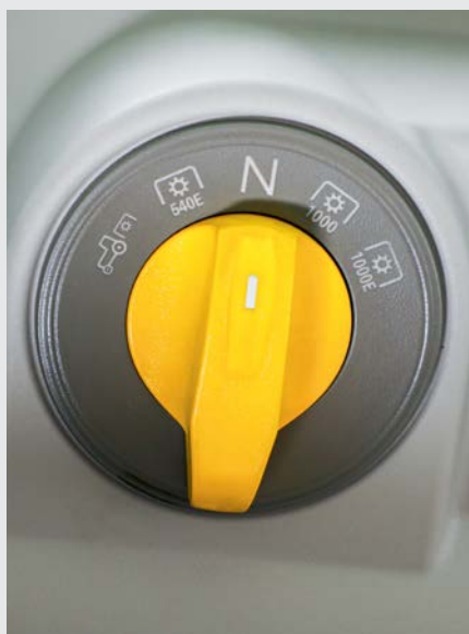
↑ Electro Hydraulic PTO selection.
